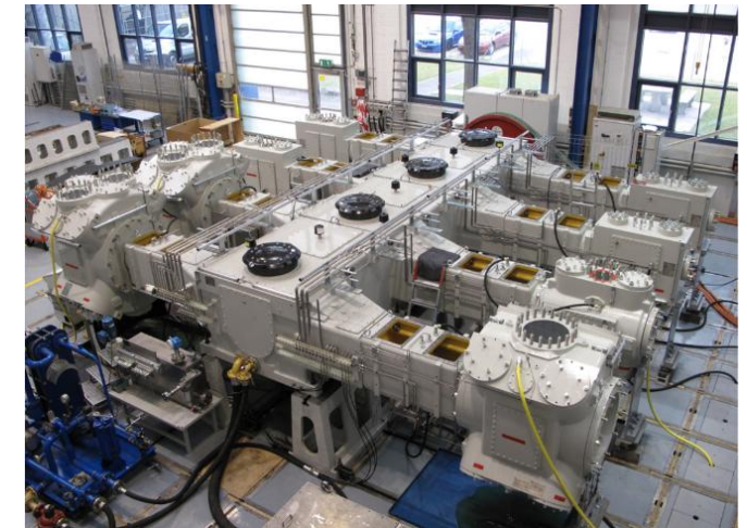
Multiservice compressor by Burckhardt Compression during MRT
